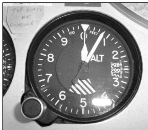
Figure 17. Barometric aircraft altimeter set at 75 ft showing a pressure of 29.87 in/Hg. Image Source: Wikimedia Commons/CambridgeBayWeather.
