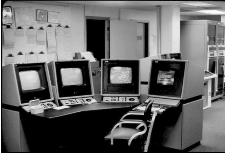
Figure 181. Early computerization showing the 1980's era Automation of Field Operations and Services (AFOS) computer terminals with the standing mainframes to their right. Image Source: NWS Buffalo Weather Office.
