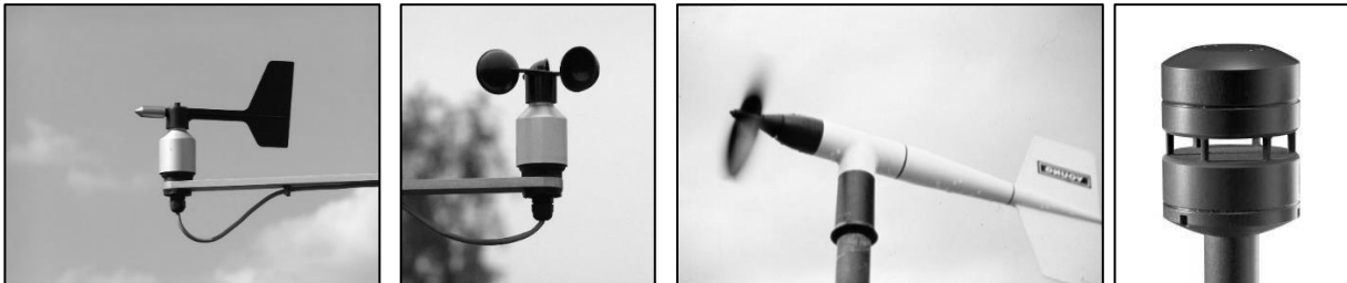
Figure 63. From left to right: wind vane (wind direction); 3-cup anemometer (wind speed); aerovane (wind direction and speed), and an ultrasonic sensor (wind speed and direction). Images source: Wikimedia Commons.
