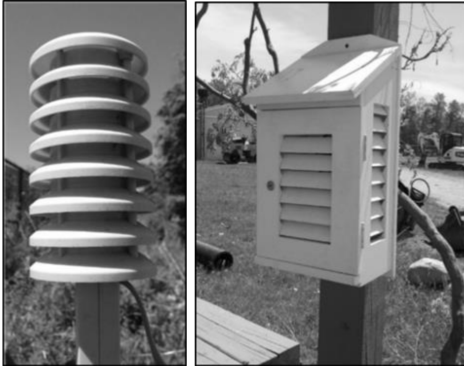
Figure 37. Thermometer shelter for electronic sensor (left) and analog thermometer (right). Usually louvered and colored white. Some shelters are aspirated (air blown across the thermometer). Image Source: Stephen Vermette.
