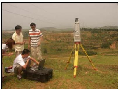
Lidar survey of digital elevation model (DEM)
