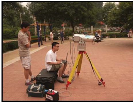
Testing of Lidar survey of solid particles in the air
