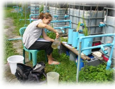
Lauren Schifferle sampling treated wastewater as part of her experiments into nitrogen transformation in constructed wetlands on the AIT campus.
